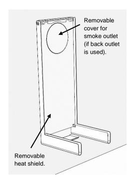
2. Place the stove on the lower rails of the bracket and push the stove in place:
