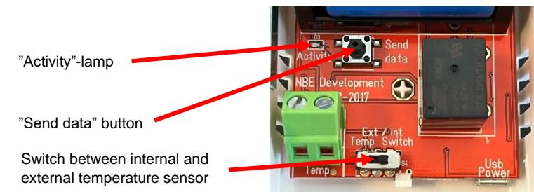
A) Remove the outer shield from the room temperature sensor and insert the batteries. Now check that the 'activity' lamp is flashing. See picture above. The room temperature sensor is equipped with an external and internal sensor. Always make sure that the room temperature sensor is set to use the internal sensor. This you can choose at the bottom of the print, where you can switch between "Ext / Int". The button must be on "Int".
